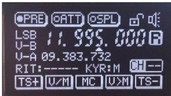
V/M: switching between the frequency mode and the channel mode;
