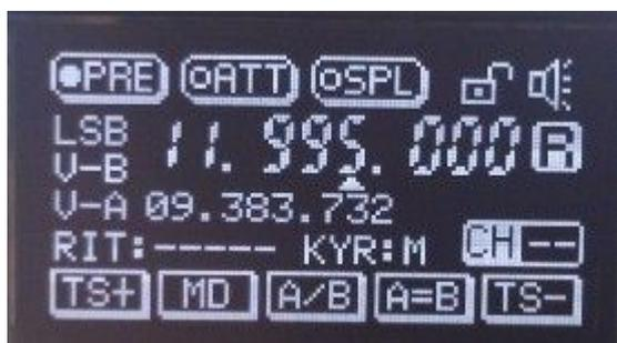
TS+: frequency step bit moving to the left for one bit;
