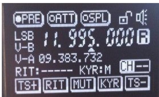
RIT: frequency tuning switch. Switching on the RIT and rotating the frequency knob for tuning frequency. When switching off the RIT, the tuning data is automatically cleared;
