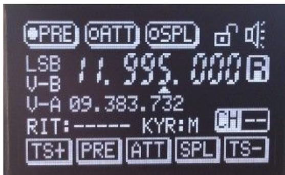
PRE: preamplifier switch. Switch on the preamplifier, a white spot will be displayed before the
